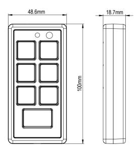
The Micro-Link packs in most features of the Opti-Link, but in a small, handy package, ideal for use in less equipped vehicles such as general purpose cars and covert vehicles. The Micro-Link offers six individual switches and a triple function 999, Arrival and Reset switch.
